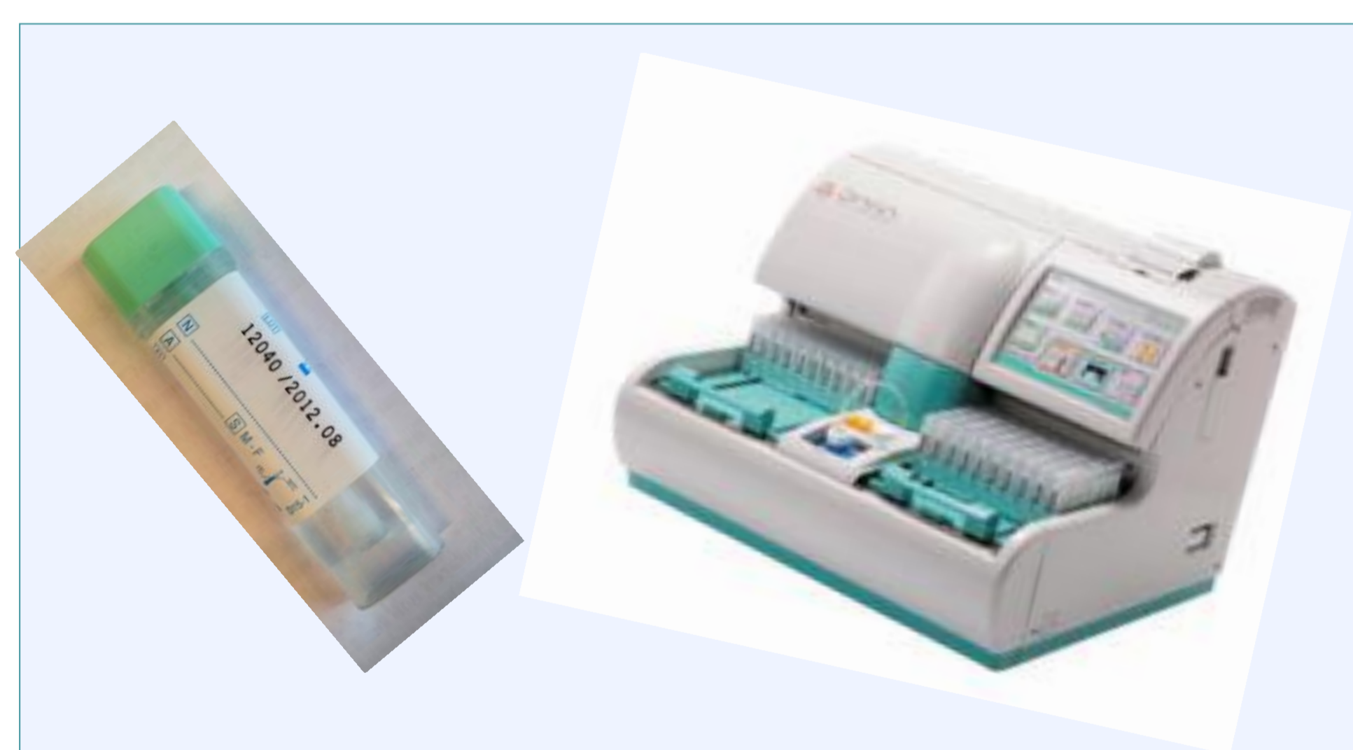
Figure 1: The OC-SENSOR DIANA analyser and sample collection bottle
